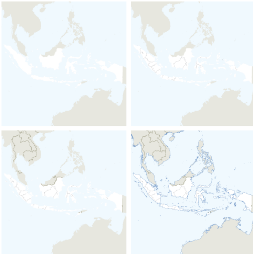
Figure 8 – The 4 maps above are meant to demonstrate the importance of appropriate data preparation of international and administrative boundaries in cartographic representation. The figure at top left displays the map polygons and each consecutive map show the polyline layers added in order from bottom (first administrative boundary) to top (coastline).
